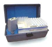
DEXSIL has developed the HydroScout System, a new easy-to-use method to quantify water in industrial and lubricating oils. Designed to be used on-site or in the laboratory, results are obtained in less than five minutes. All reagents are environmentally safe and can be disposed of in normal waste.
