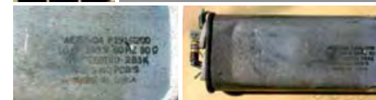
Sealed capacitors containing PCBs in high concentrations
