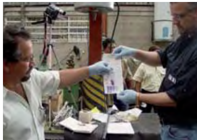
Result of oil screening using a CLOR-N-Oil kit
