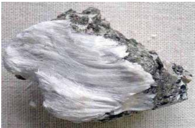
Figure 1: Asbestos (tremolite) silky fibres on muscovite from Bernera, Outer Hebrides. (Source: Aram Dulyan [3])
